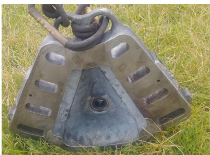
Crank pin mounting for blade crank arm
