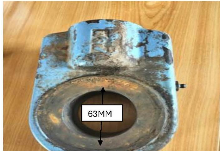
Figure 1 Clevis Bore Diameters
