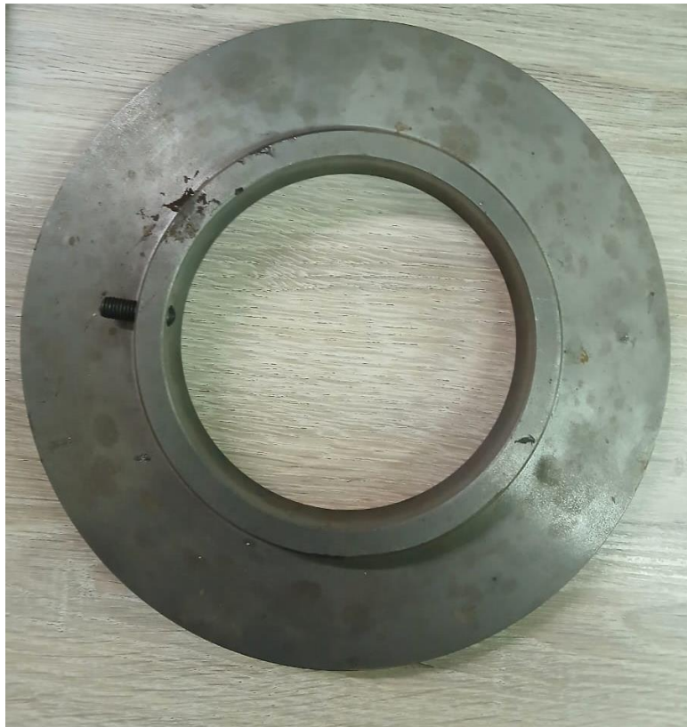
Generator bearing spacer
