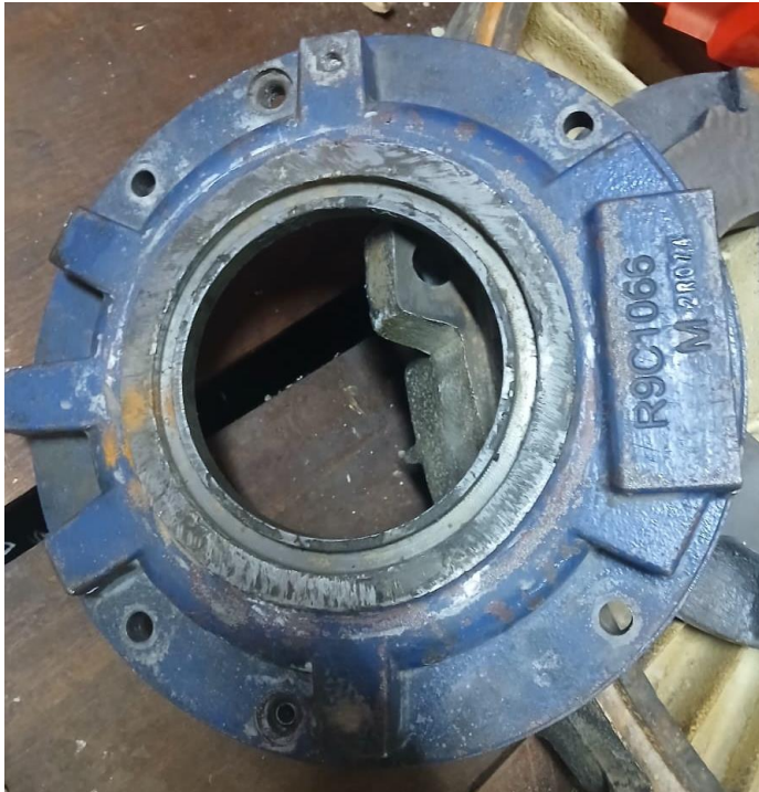
Generator bearing cover
