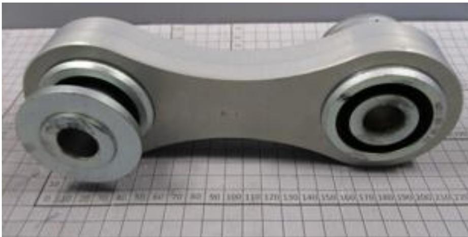
Coupling link arm and rubber bushing
