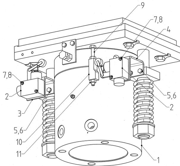
A Switching operation shall take place during insertion of the piston, just 3 mm before pressure plate get in contact with the brake cylinder. Adjusting is done by turning the roller arm of the switch.
